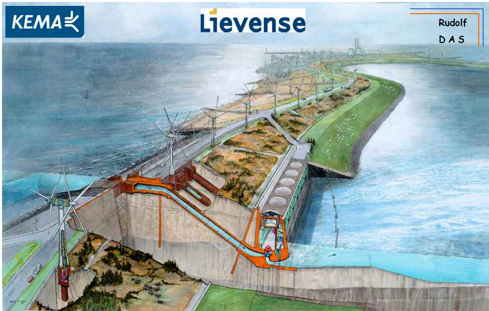
Figure 2 Cross section of the concept through the turbine
