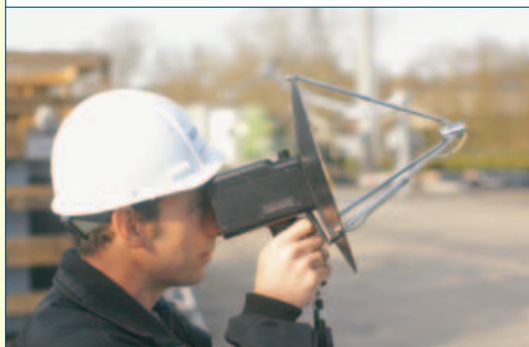
▲ A directional microphone allows the investigators to pinpoint the discharge location. Test manager Pieter Kuipers can then observe the discharges with a camera.
